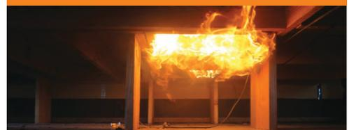
Narrow joist spacing was a condition that could result in fire growth in the under-deck area.
